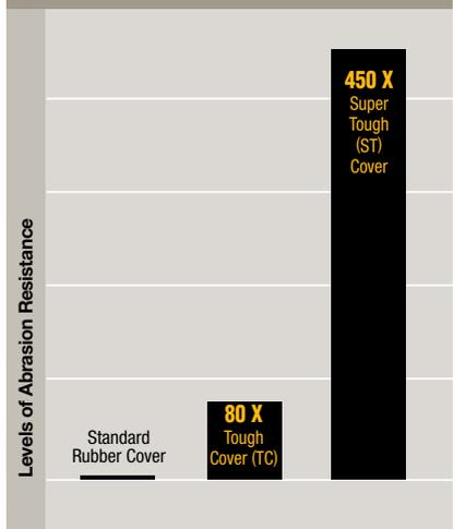
Results from the ISO 6945 metal-to-hose abrasion test show that Tough Cover and Super Tough cover hoses offer significantly greater abrasion resistance than standard rubber cover hose.
