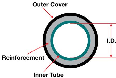
The hose size is determined by the inside diameter which can be measured or found on the layline.
