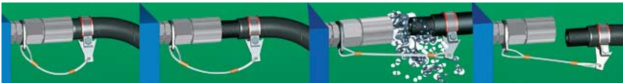
Hose Whip Restraint System limits the whipping of pressurized hose if the hose breaks free from its fitting.
