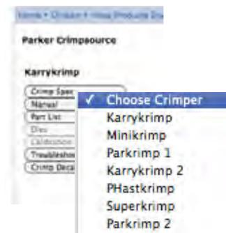
A series of drop-down menus enables users to find what they need quickly and easily. Choose your crimper and then select the hose, fittings and current specifications needed to make hose assemblies.
