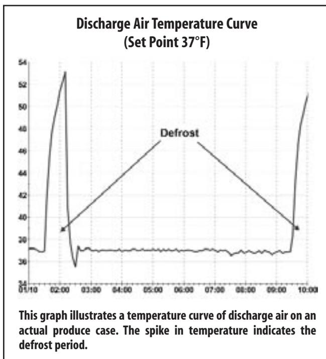
System efficiencies also can be realized with EEPRs since the coil pressure and temperature is variable and the discharge air is fixed. As the coil TD decreases with a decrease in load, the EEPR valve will throttle to maintain discharge air temperature and raise the coil pressure and saturated temperature.
