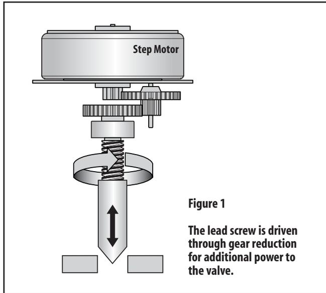
A step motor may have as many as 100 electromagnets around the rotor resulting in an angular rotation as small as 3.6 degrees between steps. The motor then drives a lead screw that converts the angular motion into linear motion with a resolution as fine as 0.0000783 inches per step. The lead screw may directly open or close a valve or the lead screw may be driven through a gear reduction for additional power to the valve (see Figure 1).
