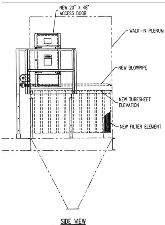
Fig. 1 Norblo converted to Pulse-Jet Collector
