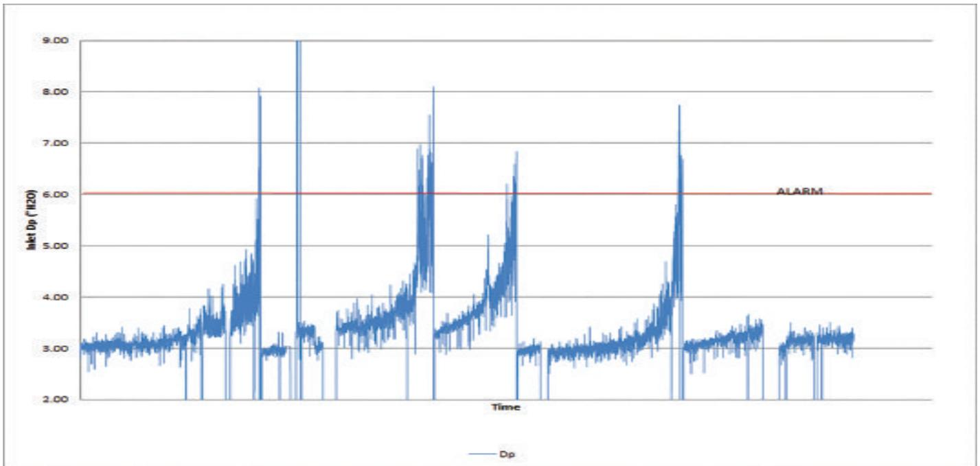
Fig. 2: The rapid dP spikes from EPA filters can trip turbine alarms and lead to unplanned outages. This side effect wouldn't be known by evaluating on filtration efficiency alone.
