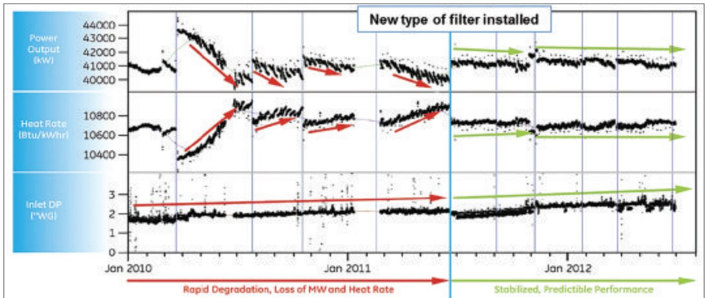
Fig. 1: This chart is one example of performance indicators to evaluate in place of filtration efficiency. This represents turbine performance, starting with, from top to bottom: MW output, heat rate, and differential pressure.
