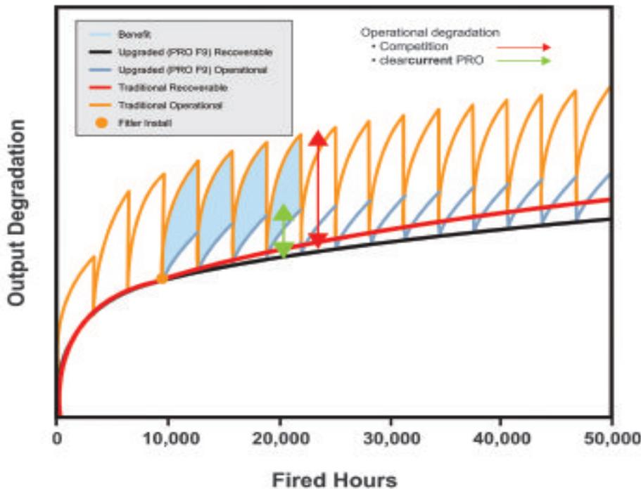
Fig. 3: The shaded blue areas indicate performance improvement by upgrading from one F9-rated filter to another, showing that all similarly rated filters are not equal in performance.
