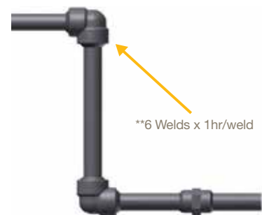
Typical 1-2" pipe with 3-socket weld fittings (6 welds).
