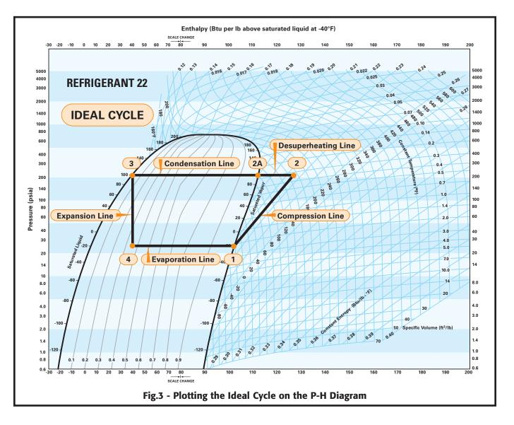
Once the system has been plotted, various data points can be read and used for the system design calculations. Admittedly, this information is not typically something the technician will need for servicing the refrigeration equipment. However, an understanding of how operating conditions affect system design, efficiency, energy consumption, and particularly compressor performance, should be of great worth to the technician.
