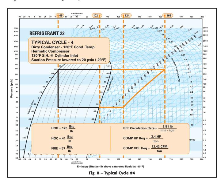
The lower the suction pressure is, the higher the refrigerant's specific volume will be, which translates into a greater compressor volume requirement. Simply reducing the suction pressure has resulted in a 30% increase in volume requirement over Typical Cycle #3.
