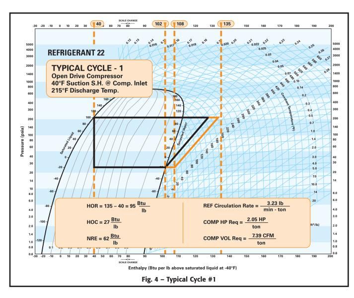
**Compressor Volume Required:** The compressor cylinder volume requirement needed to pump the RCR, in cu ft/ton. The vapor specific volume is read on the lines of constant volume.
