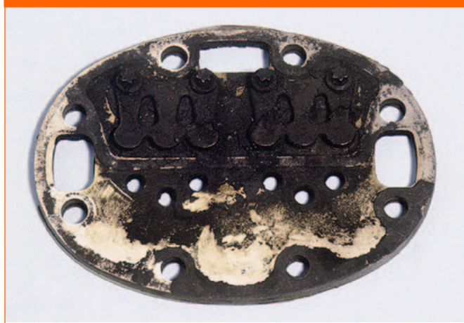
Figure 4 – Valve Plate with Oil Breakdown Deposits
