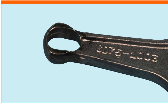
Figure 2 – Worn Wrist Pin Bore
