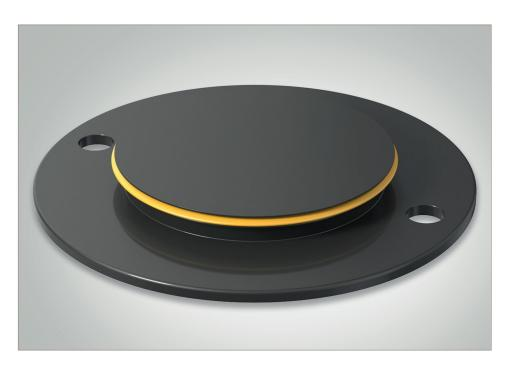
Roll2Seal® is an all-new sealing solution developed by Parker Prädifa for easy and effective sealing of bores in non-pressurized applications. The clever design combined with an equally new assembly process enables simple and accurate installation of the seal, which rolls into its seat undamaged and without a lead-in chamfer.
