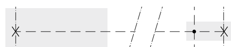
AB – Signal line plugged in inlet section and connected with tank in end section.
