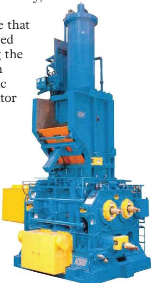
*Internal Intensive Mixer courtesy of Kobelco Stewart Bolling, Inc. Hudson, Ohio*
