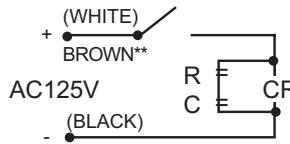
CR: Relay coil (under 2W coil ratings)
