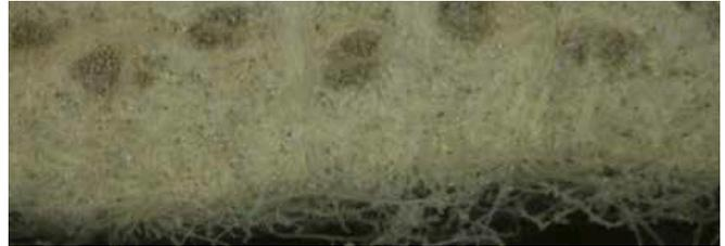
Bag 2 cross section is packed with dust.
