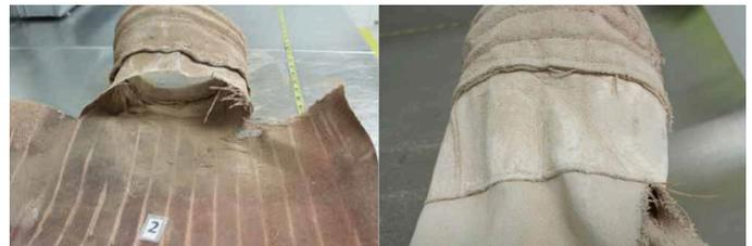
Top interior with apparent thermal damage. Media exhibited stiffness/brittleness in this area.
