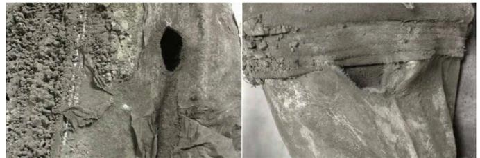
**Bag #1.** Circular hole along filtration side of the bag. Hole appears to have been formed from the exterior. Large chunks of contaminant adheres to the outside of the bag. Large areas of peeling membrane.
