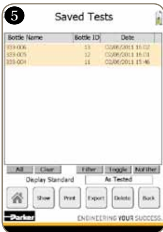
Export results: Highlight the test result(s) you would like to export using the stylus.
