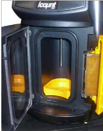
Fig 4. The IBS oil sampling probe automatically lowers into the bottle once the test begins.
