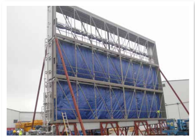
Every evaporative cooler is run through a first-piece qualification performance test before it is delivered to the customer. Above, an evaporative cooler for a GE 9FA turbine is put to the test.
