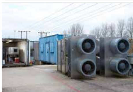
Our outside test rigs allow us to evaluate filters for up to 6 months and measure a variety of factors, including initial DP, fractional efficiency, and reaction to mist and fog.
