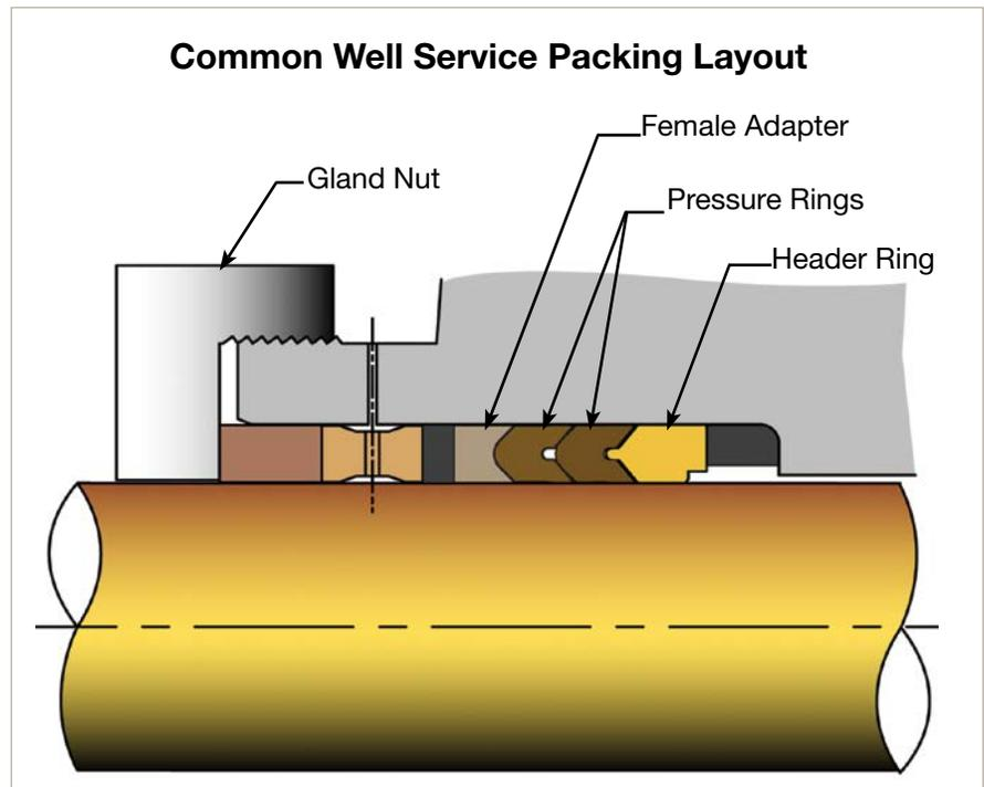
NOTE: Parts in the stack may vary based on pump model. Refer to the pump manufacturer's parts list for stack arrangement.
