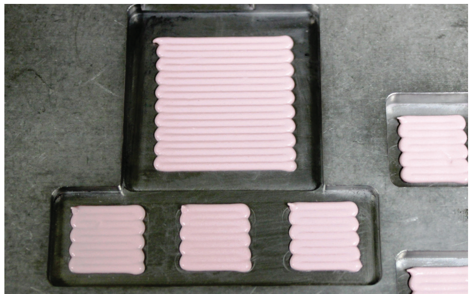
Figure 4: Multiple location casting
