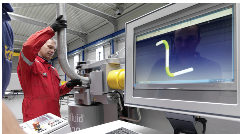
CNC controlled pipe and tube benders in a shop environment for pre-fabrication
