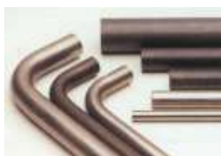
Tubes and Tube Bends Seamless EO tubes and tube bends according to DIN 2391. Material: St 37.4 steel and 1.4571/1.4541 stainless steel
