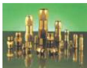
Check Valves Check valves for in line mounting or cartridge systems. Several unique features (double seat, no seal, guided poppet, oil retention groove in the poppet and poppet-guide cushion) that ensure years of trouble-free operations.
