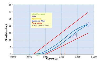
The above curve illustrates the relationship between flow rate at a particular current input signal at a constant inlet pressure for a proportional valve. The key characteristics measured are shown in the legend.
