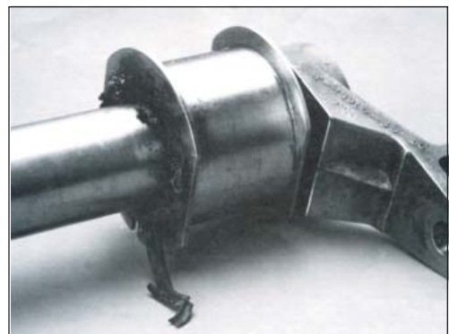
Figure 7 – Unacceptable fatigue and fluid contamination on Turboprop Engine Mounting (DeHavilland Dash 8)
