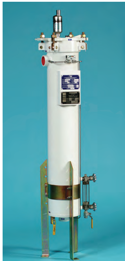
Vel-Max ® Filter Vessel, VX-2, showing optional leg assembly, differential pressure gauge, sight glass assembly, and air eliminator.
