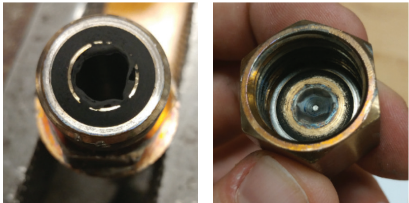
Figure 3 – Seal-Lok CNG after passing Bonfire Test
