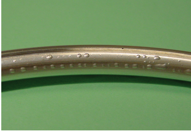
Figure 2: Blisters seen on a standard silver plated seal after 500 hours in air at 400°F (204°C).
