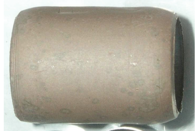
Figure 3: Silver-indium sample exhibits virtually no blisters after 500 hours in air at 1150°F (621°C).
