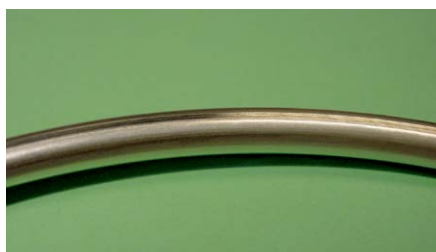
Figure 2: Parker Hannifin's Silver-Indium diffused plating
