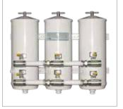
All double and triple manifolded assemblies have steel ball valves to allow the isolation of each unit so you don't have to shut the engine down to service the filter. The manifold pipes are threaded at each end, so once installed on the engine, fuel can flow from the left or right—just cap the ends you do not use.
