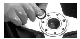
2. Then from the back of the motor housing, remove the shaft seal.
