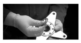
6. Reinstall thrust bearing package with washer on bottom and bearing on top.
