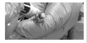
Mark shock valve in the same color that was used to mark the housing and plug.
