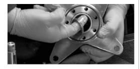
Remove shaft seal, backup ring and backup washer.
