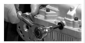
3. Loosen the shock valve using a 5/16" hex wrench on the reverse side.
