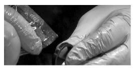
Shaft Seal Installation Procedure for HTE w/ Date Code on or after 25 216 is on the next page. Using the lubricant provided in the seal kit, grease shaft seal before installing.
