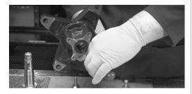
1. Using a screwdriver, press from the front of the motor housing, releasing the shaft seal.
