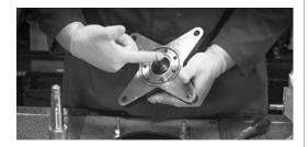
Install backup ring, backup washer and shaft seal.
