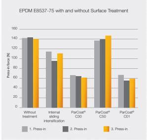
Even when the same O-ring is repeatedly installed, the assembly forces remain at a consistently low level.
