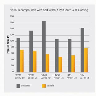
Press-in forces required for installation of standard connectors on automotive air conditioning systems with ParCoat® C01-coated and uncoated O-rings.
