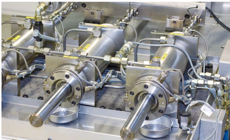
Figure 1: Endurance test rig according to ISO 7986
