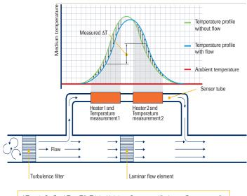
$\Delta T = k.C_{m} \mathcal{O}_{m} \Delta T = T2-T1$  in Kelvin  $C_{m} = \text{specific heat } \mathcal{O}_{m} = \text{mass flow}$
