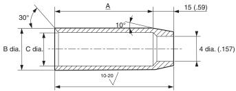
full length of O.D. no tool marks or scratches permissible with a smooth intersection between 10° chamfer & dia. "B".
