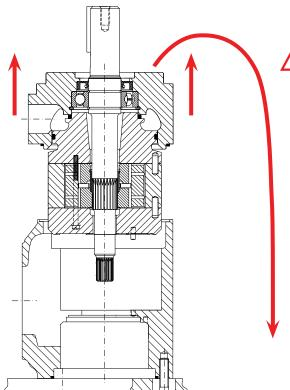
P1 cartridge will come with the front cap / shaft assembly.
