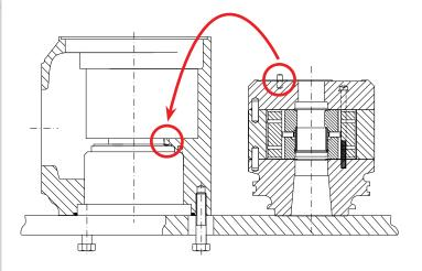
Check if the dowel pin is in its position in the housing by trying to rotate the cartridge.
