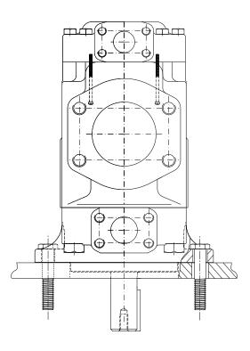
Two bolts will help to unscrew the 4 pumps bolts.
