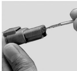
1. Grab the crimped contact approximately 25 mm behind the contact barrel.
