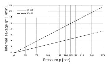
Do not operate pump more than 5 seconds at any speed or viscosity if internal leakage is higher than 50% of theoretical flow.
