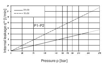
Do not operate pump more than 5 seconds at any speed or viscosity if internal leakage is higher than 50% of theoretical flow.
