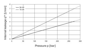
Do not operate pump more than 5 seconds at any speed or viscosity if internal leakage is higher than 50 % of theoretical flow.
