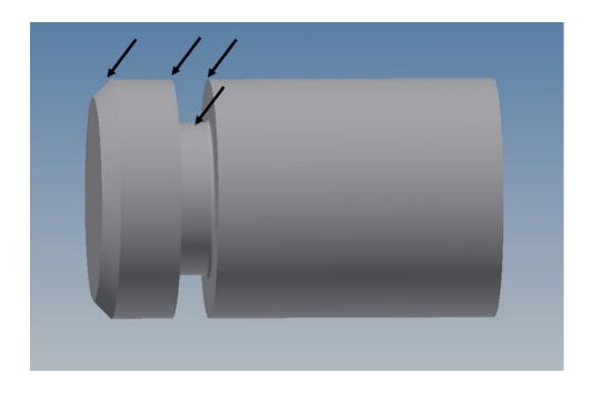
Inspect the piston and piston groove for sharp edges, gouges, dirt or debris that could damage the rubber expander.
