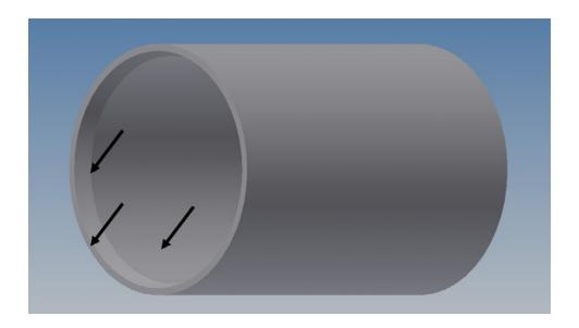
Inspect the bore and the bore lead-in chamfer for nicks, burrs with sharp edges, gouges, dirt or debris that could damage the plastic seal ring.
