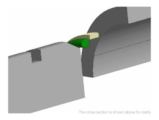
Apply a thin film of hydraulic fluid to the expander, seal ring, bore and piston to ease assembly. Using both hands, stretch the rubber expander over the piston and slide into the groove. Exercise caution to not use any tool with sharp edges to damage the expander or transport debris onto the seal.
