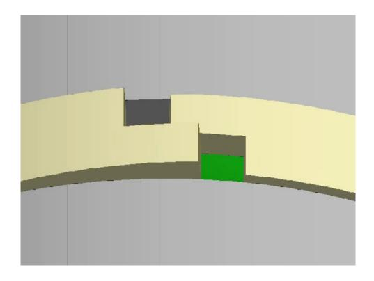
Compress the seal ring so that the step joint is fitted properly.
