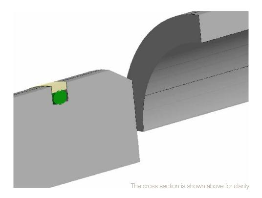
Lubricate all seals and install the piston into the bore so that the plastic step joint is approximately opposite the cylinder fluid port. Carefully, slide the piston assembly into the bore making sure that the plastic ring remains in the piston groove and is not damaged. Fill with system recommended fluid and follow the cylinder manufacturer's system final assembly instructions.
