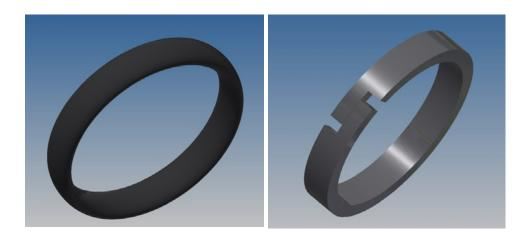
The ChemCast® Seal consists of a rubber expander and a plastic seal ring with a step cut. Do not modify these component parts in any way. Grinding, trimming or shaving of any surface of the seal ring or expander will adversely affect the sealability of the seal assembly.
