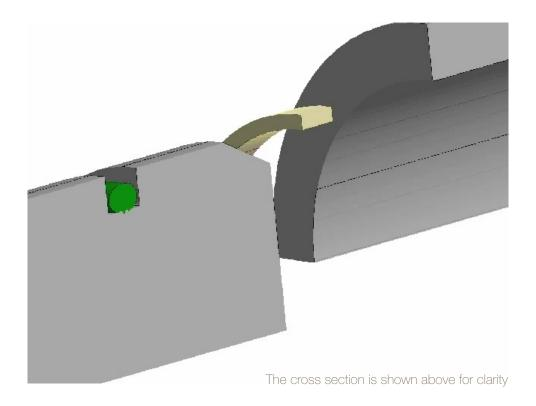
Slide the plastic seal ring over the piston and position over the expander in the piston groove. Make sure to expand the plastic ring diameter only enough to slip over the piston diameter. Excessive stretching of the seal ring will weaken the seal ring. Exercise caution to not transport debris onto the seal components.
