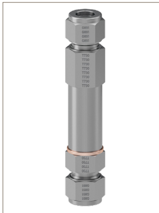
Parker Bestobell Cryogenic Thermal Relief Valve in Full Stainless Steel (12mm Two Ferrule A-LOK® Inlet and Outlet connections)
