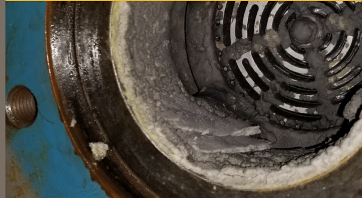
Actual salt build-up inside of compressor cylinder before installing Gemini vessels
