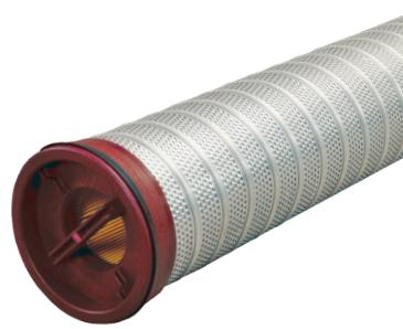
The XtreamPure, Series XP-C, is a large 6" diameter cartridge designed to filter liquid from inside-to-outside. This design has several advantages. It allows for high flow rate capability within a single cartridge so fewer cartridges are needed compared to traditional 2.5" and 3" diameter designs. It keeps contaminants trapped within the cartridge, so the vessel remains clean. The cartridge includes a handled end cap with patented chevron seal technology to provide an absolute
