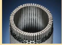
Heavy duty coalescing filter with proprietary media saturant designed to remove high loading of liquid aerosols and fine particulate from natural gas. High flow, low pressure drop. First stage for pipeline gas or second stage for wellhead gas.
