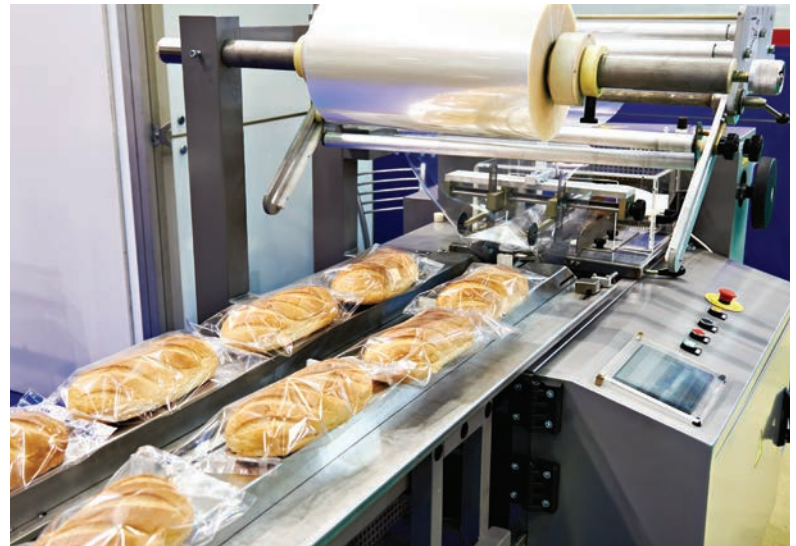
HFFS, (Flow wrapper packaging bakery products).
