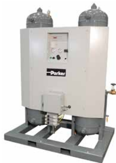
Pressure Swing Adsorption (PSA) nitrogen generators use a Carbon Molecular Sieve (CMS) material inside a vessel that contains pressurized air to draw off the nitrogen molecules. Photo courtesy of Parker Hannifin
