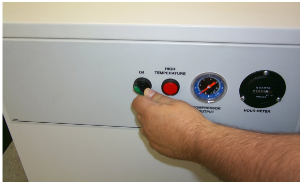
Figure 19 Compressor Power OFF Switch
