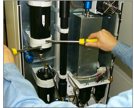
Figure 37 Tri-Gas Changing In-Line Filter
