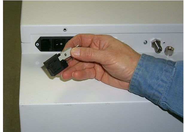
Figure 10 Tri-Gas Generator Voltage Selection
