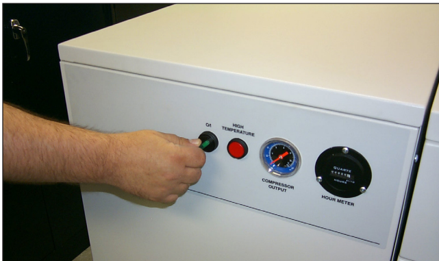
Figure 15 Compressor Power On Switch
