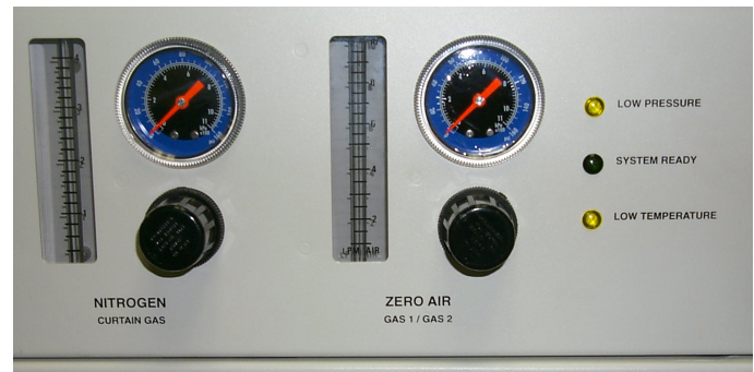
Figure 18 Gas Generator LED Indicators
