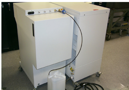
Figure 13 Tri-Gas Drain to Disposal Container
