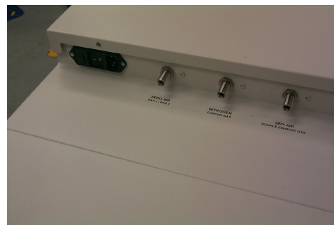
Figure 14 Three Outlet Gas Fittings
