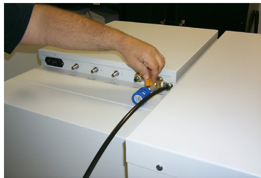
Figure 21 Tri-Gas Generator Depressurizing - Open Valve
