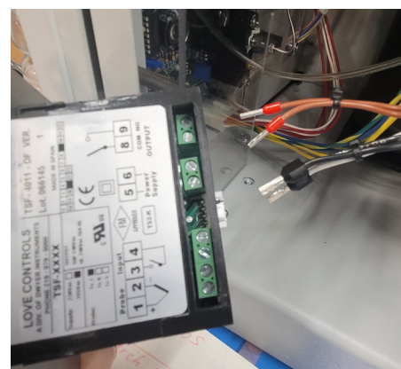
Figure 8 - Limit Controller Wiring
