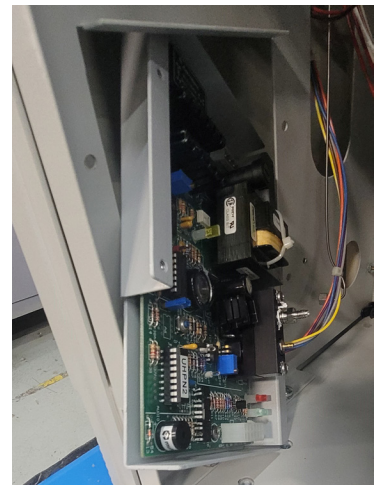
Figure 5 - Removing PCB Assembly from the UHP Chassis
