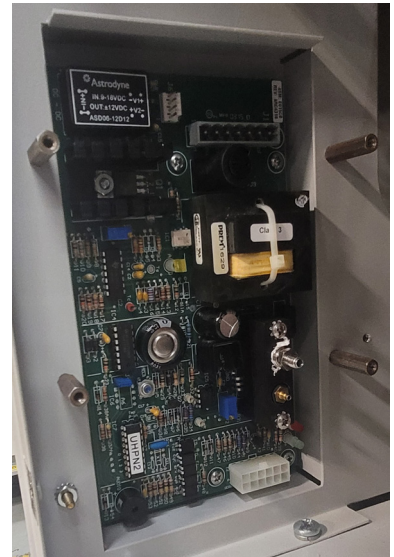
Figure 4 - PCB with connectors and tubing removed
