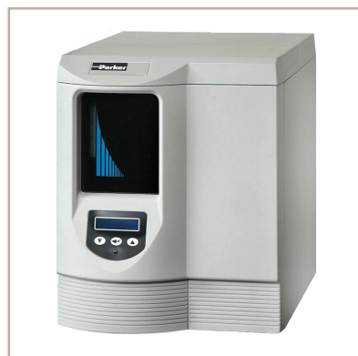
Fig. 1. Parker Hydrogen Generator produces up to 1,300 cc/minute of 99.99999+% pure fuel and carrier gas at up to 175 psig.
