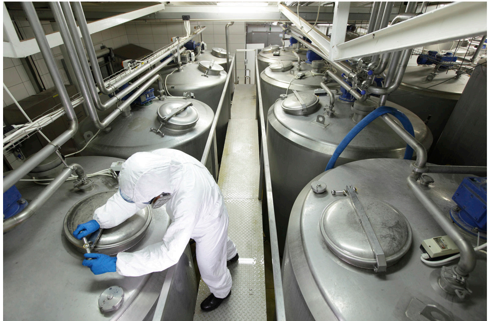
Large tanks such as these are used to store edible oils.
