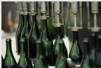
Nitrogen blanketing is being used in the wine bottling process.
