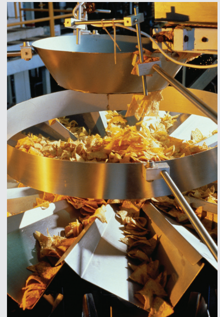
Snack items such as chips are to be slipped into packages, after which the equipment shoots a stream of carefully controlled amounts of nitrogen into the package to eliminate the possibility of spoilage.
