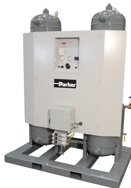
Pressure Swing Adsorption (PSA) nitrogen generators use a Carbon Molecular Sieve (CMS) material inside a vessel that contains pressurized air to draw off the nitrogen molecules.
