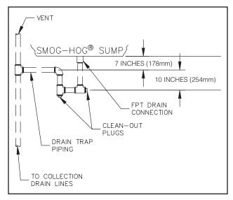
Notes: Main drain line should be sufficiently sloped, 1.5 inches (38mm) diameter and vented. All plumbing should conform with all state and local codes.
