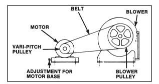
Figure 10 Motor/Blower Schematic
