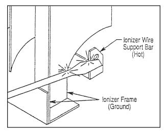
Figure 5 Grounding the Ionizer
