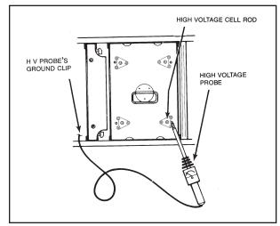
Figure 12 Checking Ionizer Voltage
