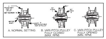
Figure 11 Motor Pulley Settings
