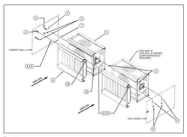
Figure 14 Properly Aligned SHN Assembly
