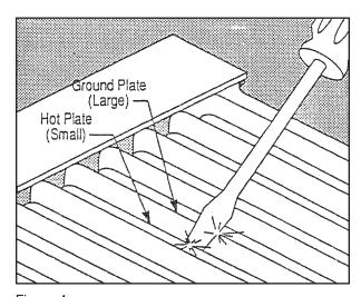
Figure 4 Grounding the Collection Cell
