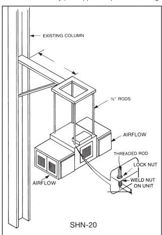
Figure 2 Column Mounted Unit
