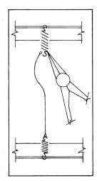
Figure 8 Attaching New Ionizer Wire
