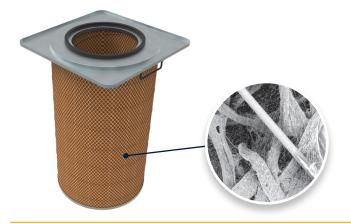
Protura DH nanofiber technology is a fine surface membrane applied to the filter substrate that prevents dust from penetrating into the filter pores and plugging the filters. Surface loading minimizes pressure loss and improves filter cleaning, extending filter life.
