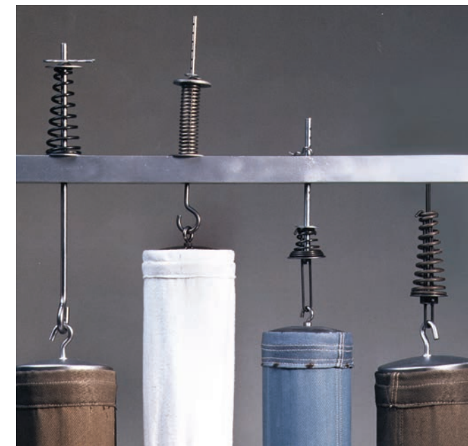
Figure 14. Tensioning assemblies allow the fabric enough movement to clean down, yet control filter bag collapse.
