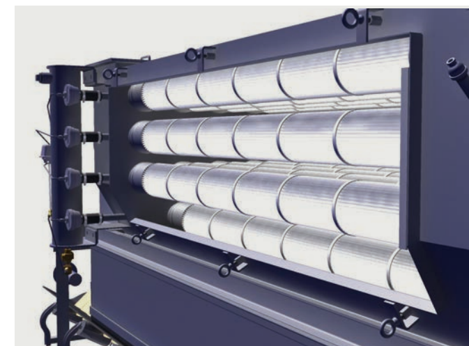
Figure 33. Horizontal collector with easily replaceable pleated filter elements.
