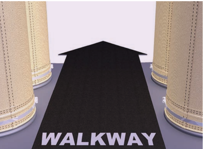
Figure 16. Proper seam orientation as viewed through the access door, reducing the potential for bag-to-bag abrasion.
