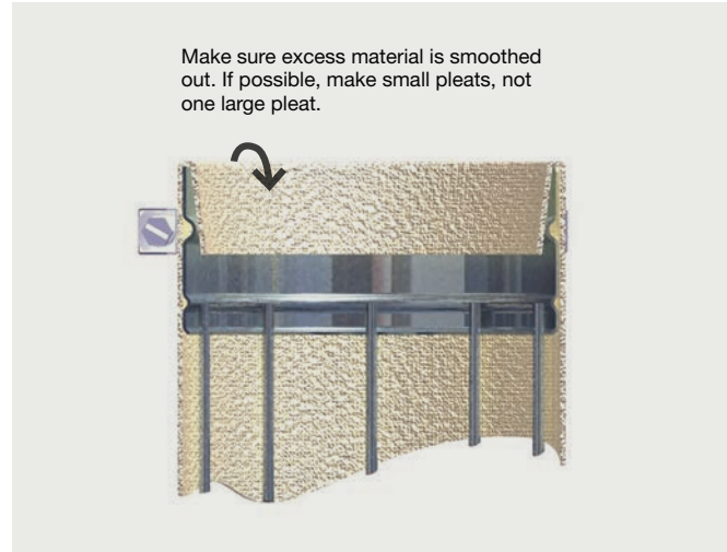
Figure 9. Check for smoothness around the edge when bag flanges or cuffs fold over the top of the cages.
