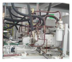
This turbine starter system utilizes a Gold Cup P11P pump with a T6 vane pump mounted to the rear to drive a bent axis motor.
